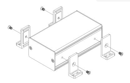
**Step 2** Use self-drilling screws to fix the product on a platform
