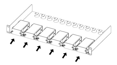
**Step 4** Install the rack in a cabinet
